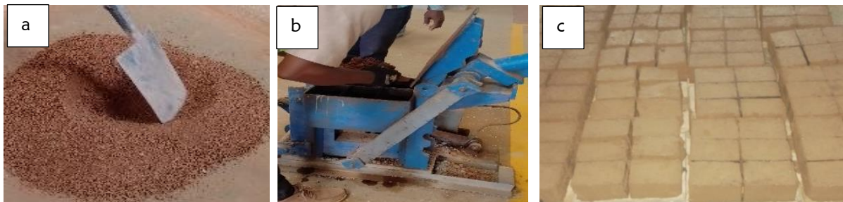
Figure 3: Preparation of bricks: (a) mixing of materials, (b) moulding of bricks, (c) drying of bricks
